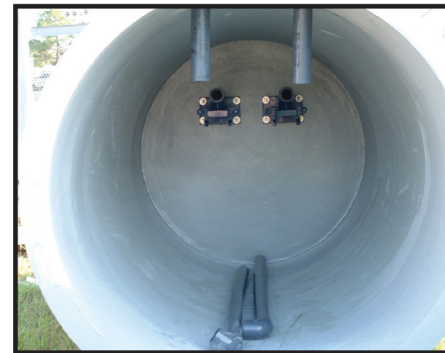
Fabrication of a 48" x 10' wet well piped with 2" SCH-80 PVC and BERS-200 pump discharge bases.
